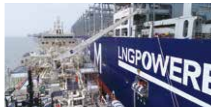
Demonstration of ship-to-ship loading operation with an LNG-fueled containership
