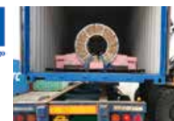
Transport of steel coils using MOL COIL-PORTER®
