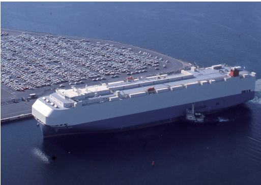
A car carrier with a capacity of 6,400 units
